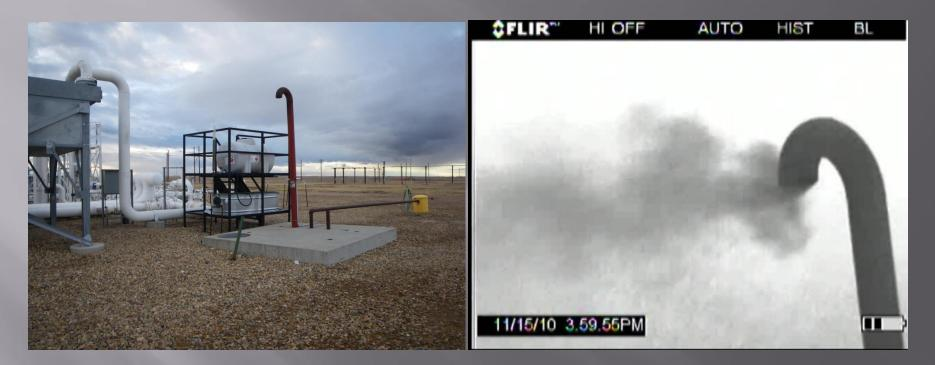
Compressor distance piece oil sump at a natural gas compressor station
