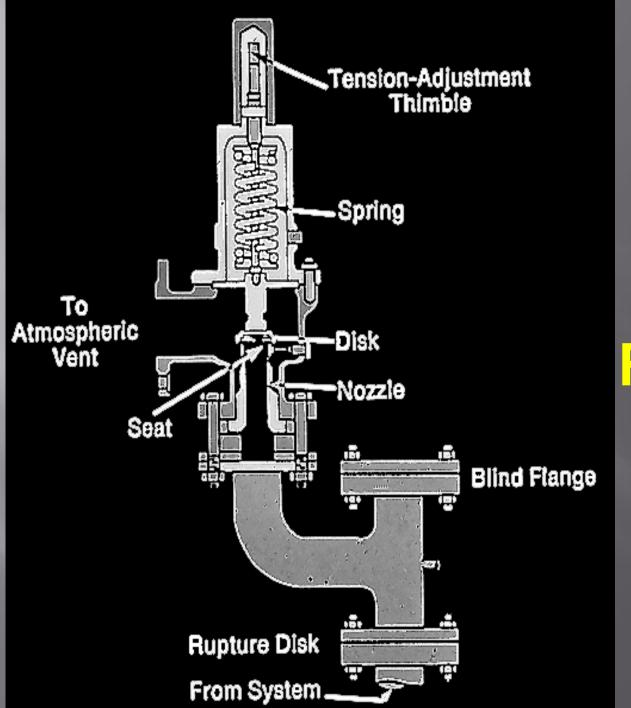
PRV with Rupture Disk
