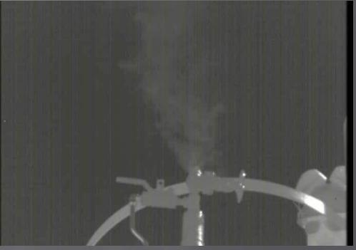
New "alternative work practice" promulgated to allow the use of optical gas imaging as a replacement for method 21
