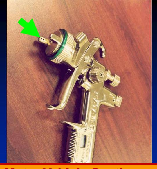
Motor Vehicle Coating – High Volume Low Pressure (HVLP) Spray Gun
