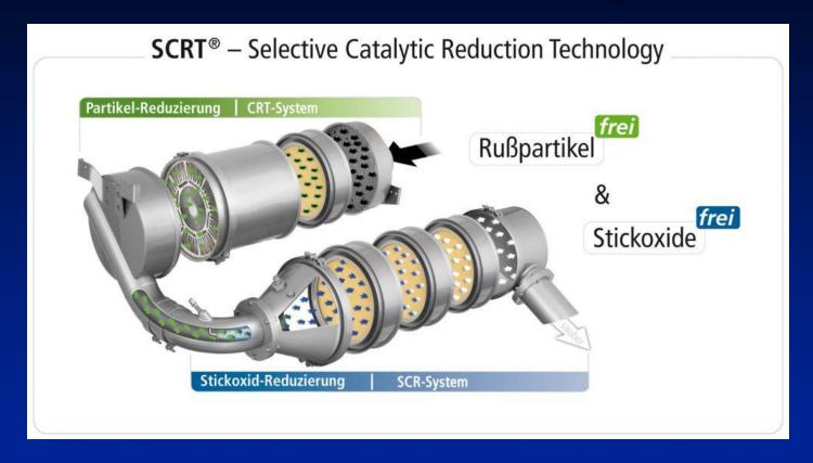
$2 \text{ NH}_3 + \text{NO} + \text{NO}_2 \rightarrow 2 \text{ N}_2 + 3 \text{ H}_2\text{O}$
