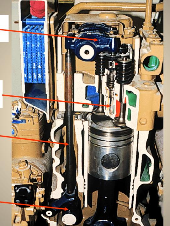
Diesel Engine Cross-Section
