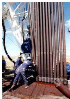
Tripping Out Pipe
