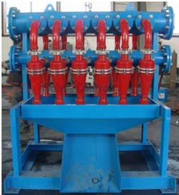
De-Silting Cyclones over Mud Tank
