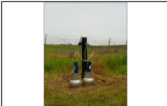
Compendium Method TO-15 Application for Monitoring VOCs at the perimeter of a MSW Landfill 61
