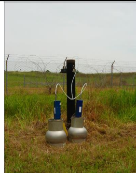
Compendium Method TO-15 Application for Monitoring VOCs at the perimeter of a MSW Landfill 60
