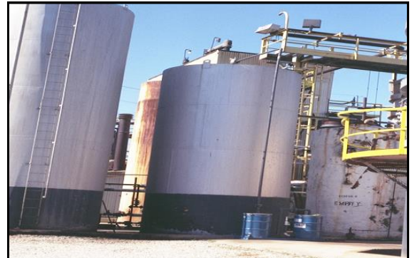
Non-Regenerable Carbon Adsorption Drums controlling mercaptan odors from re-refined crankcase oil product 4 - 106
