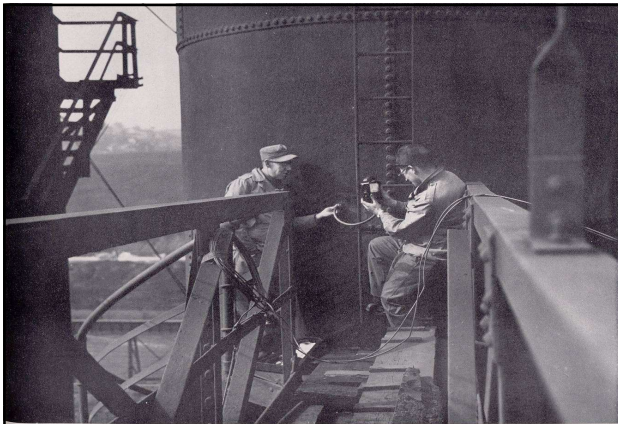
Stack Measurement in Donora (Circa 1948) 1 - 3 Measurements of airflow in study of stack effluents.
