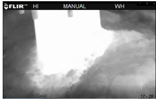
Leachate Extraction Well Riser Fugitive Emissions
