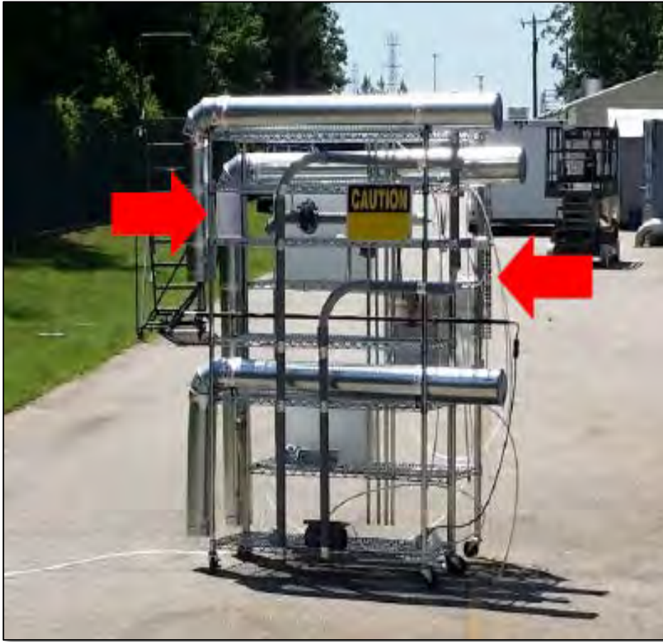
Figure 3-42. ERG Controlled Leak Simulation Platform
