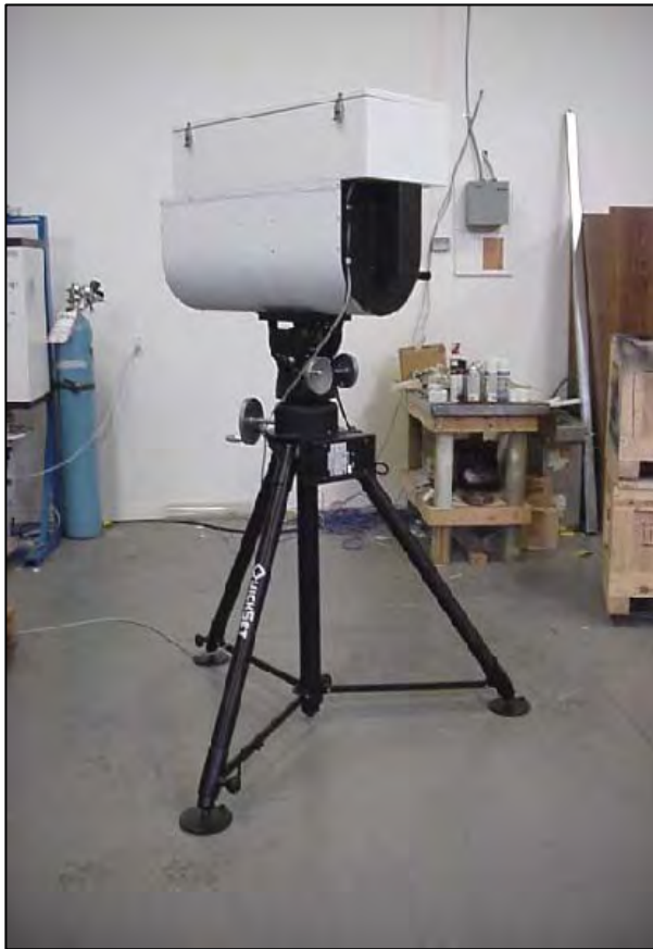
Figure 2-6 Typical telescopic FTIR Transmitting and Detection Unit
