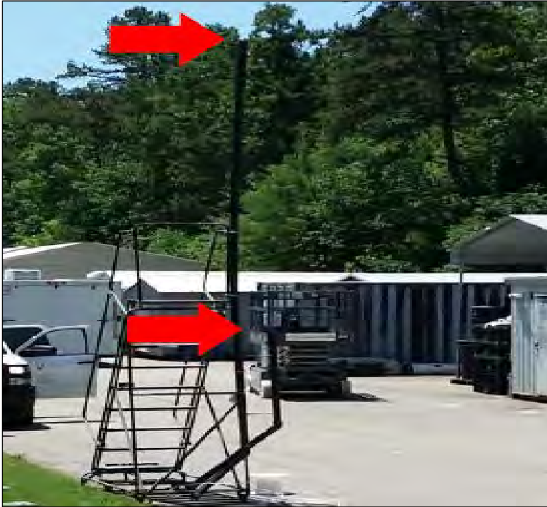
Figure 3-41. High/Low Controlled Gas Release Platform
