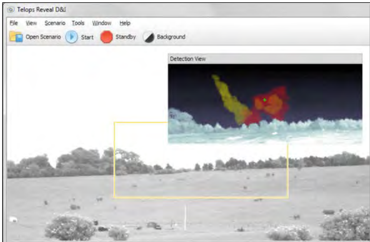
Figure 3.38. Example Telops Software Output Where the Detection View is the Total Radiance with the Gas Cloud Highlighted in False Color.
