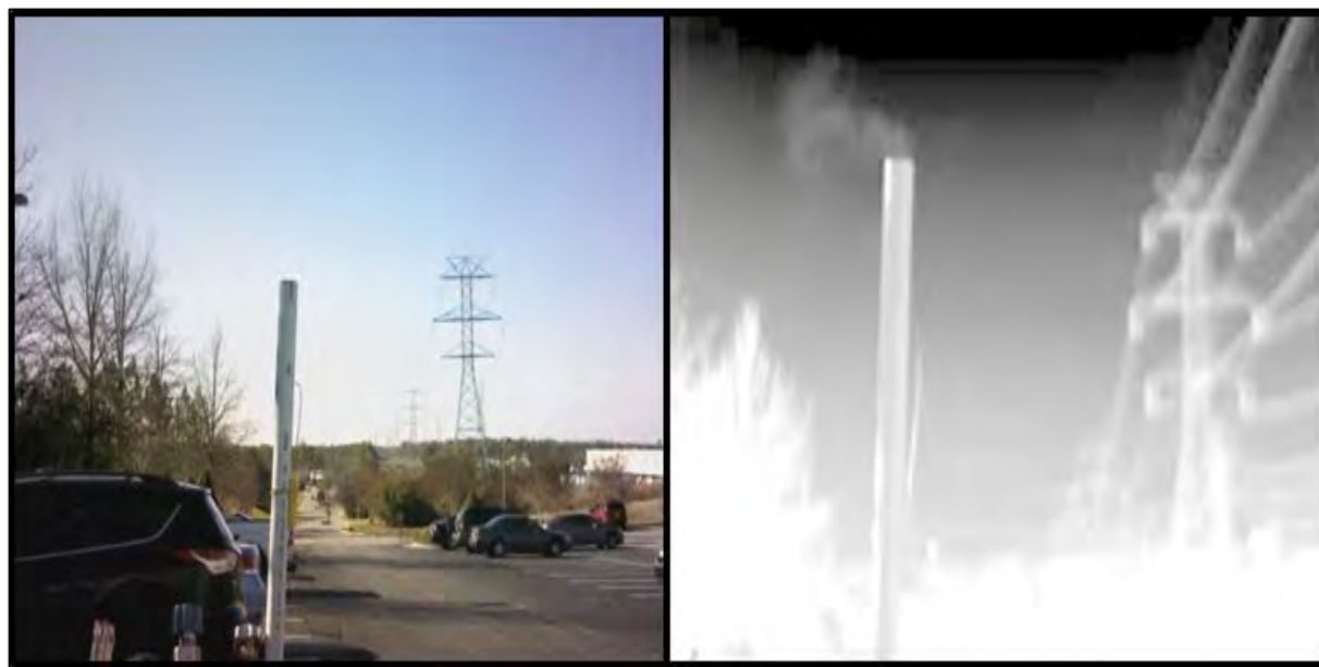
Figure 2.23. Image of a Controlled Gas Release where the Gas is Warmer than the Background.
