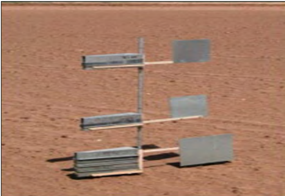
Figure 3.49. BSNE Sampler Shown Sampling in the Field. 7
