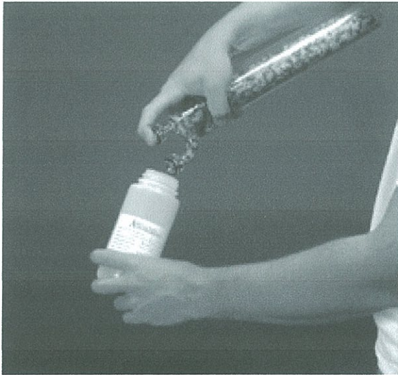
Figure 2-28 Recovering Silica Gel for Weighing
