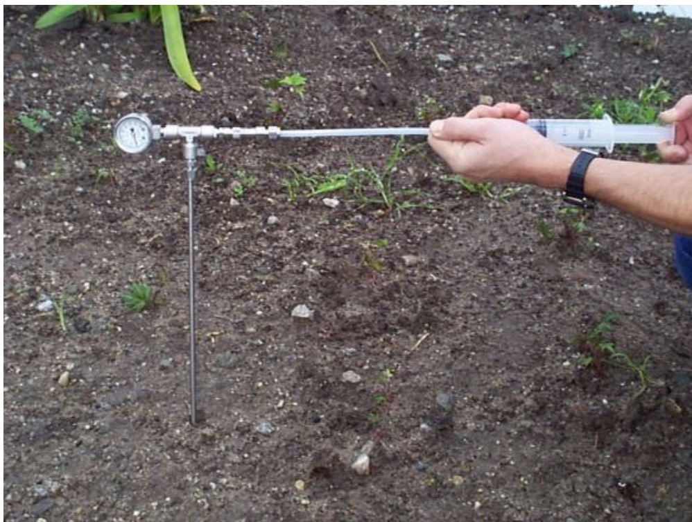
Figure A-10. Application of Syringe Monitoring for VOCs at a MSW Landfill.
