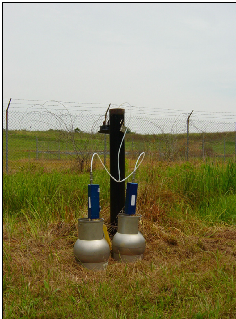
Figure A-17. Compendium Method TO-15A Application for Monitoring VOCs at the perimeter of a MSW Landfill.
