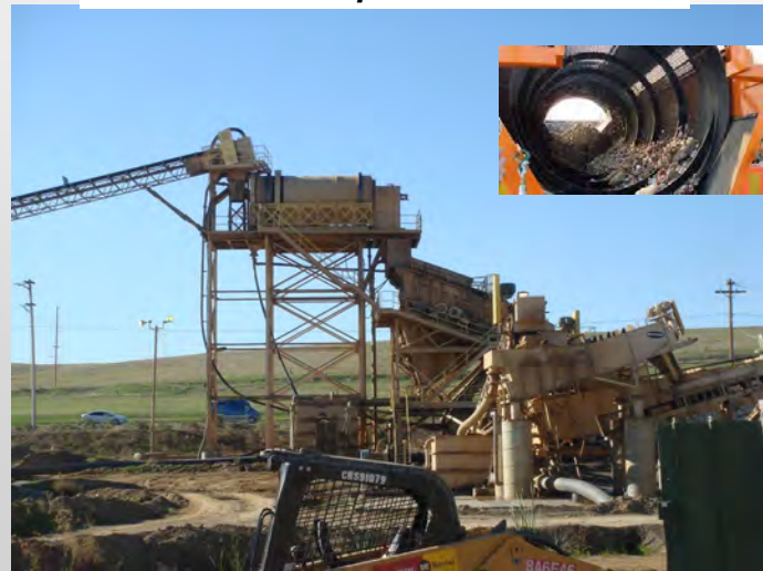
Wash Plant w/trommel screen
