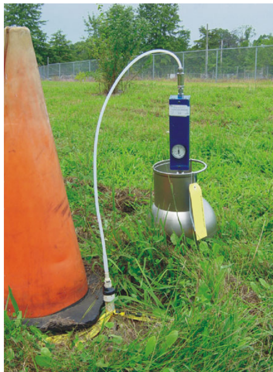
Landfill Gas Sampling at a Temporary Gas Monitoring Probe
