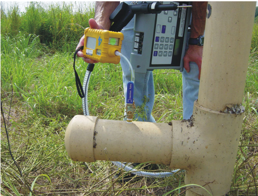
Landfill Gas Screening at a Passive Vent
