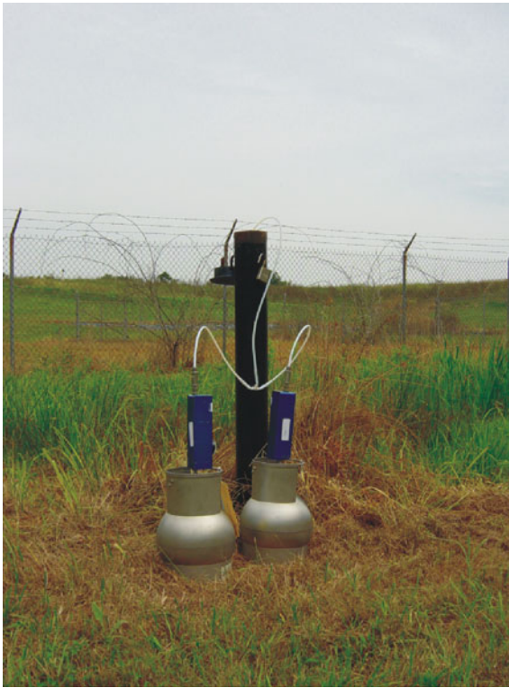
Landfill Gas Sampling and Duplicate Sampling at a Perimeter Gas Monitoring Probe
