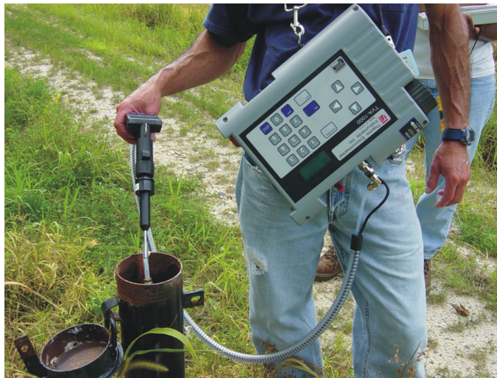
Landfill Gas Screening of a Perimeter Gas Monitoring Probe
