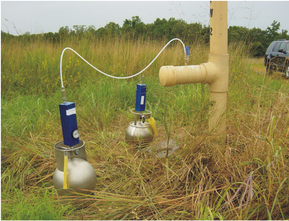
Landfill Gas Sampling and Ambient Air Sampling at a Passive Vent
